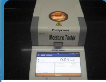
Polymer Moisture Content Tester
